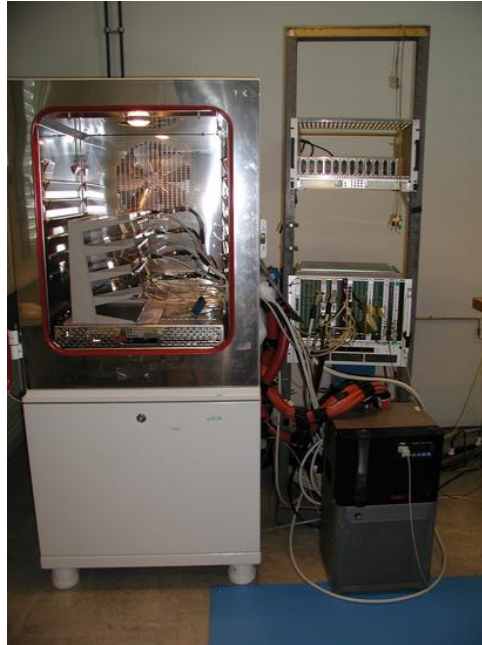
Figure 27: The test setup for module quality assurance at CERN - 4 modules inside a climate chamber which allows “cold” tests of the modules.
