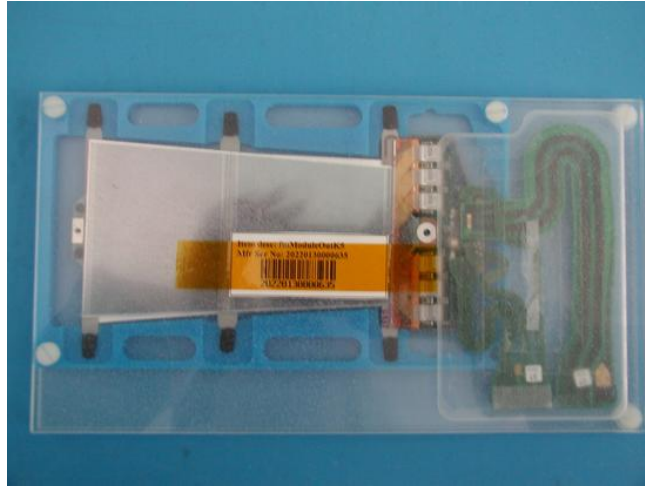
Figure 26: A module that passed the electrical readout tests at the University of Geneva, packed in a transport box before being shipped from the University of Geneva to CERN.
