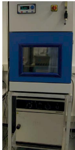
Figure 6: The climate chamber used for thermal cycling of the modules
