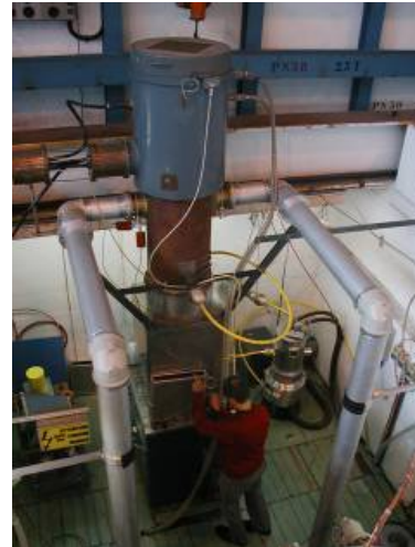
Figure 5: The 2 MW amplifier; in the right corner its driver is visible.
