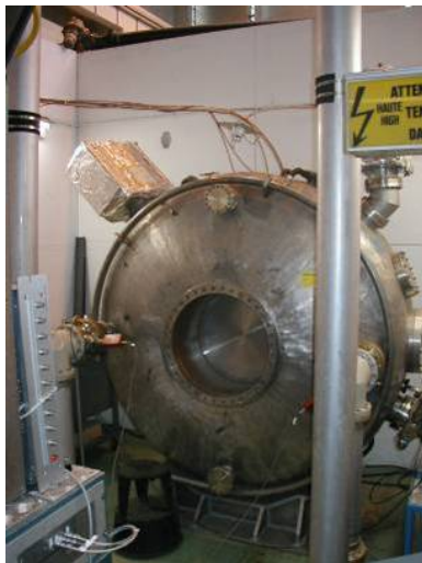
Figure 4: The 88 MHz test cavity.
