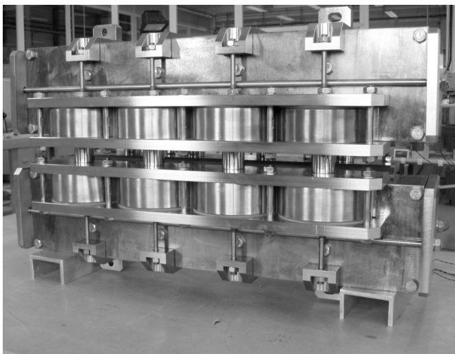
Fig. 6. Undulator full scale prototype assembly: two yoke, eight coils.
