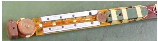
Fig. 9. Superconducting wire loop in the device for contact resistance measurement
