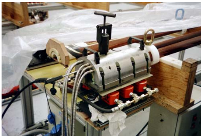
Fig. 2. Example of “minor tooling” for cold mass production.
