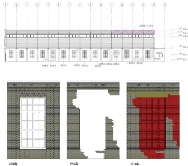
Figure 7. The wall damage documentation and partial inner wall changes of machinery engineering workshop, Dagu Dock of Beiyang Navy (International Research Center for Chinese Cultural Heritage Conservation of Tianjin University, 2014)
