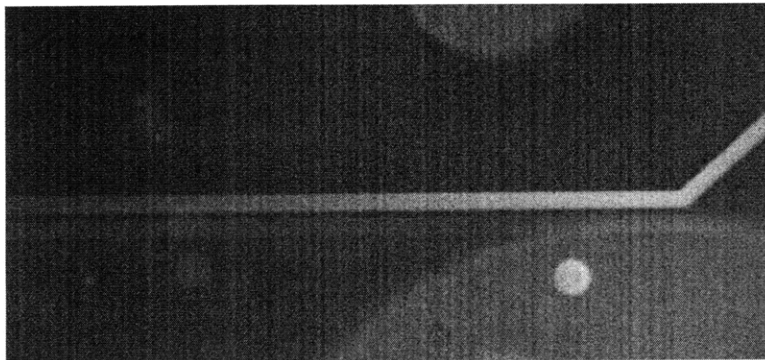
Figure 4c: Two interconnected microchannels are shown in this picture; the channels are coated with anti-RPE antibodies. A 100ng/mL RPE solution was injected from the top right corner, and exits in the lower right corner. This picture is taken after the channels has been flushed with PBS 1x, and shows a decrease in intensity along the sample flow path. This reflects the depletion of RPE molecules in the sample solution along the channel.
