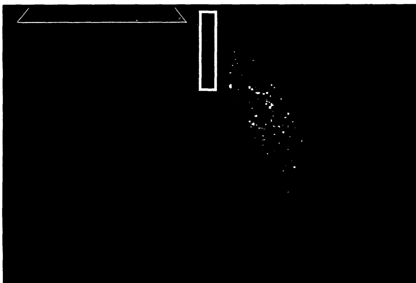
Figure 4.5: ROI (276, 9) – (296, 117) superimposed on two-second image of indolene fuel with camera triggered at 45 CA aTDC and focussed on valve centerline plane.
