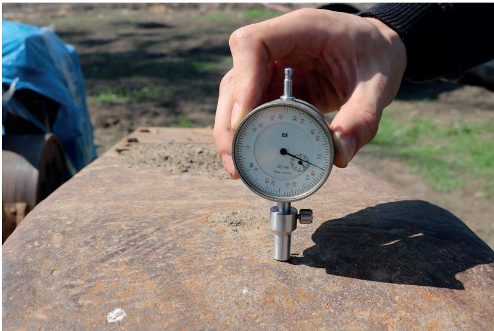
Fig. 4. The device for measuring the depth of corrosion pits (accuracy 0.01 mm)
