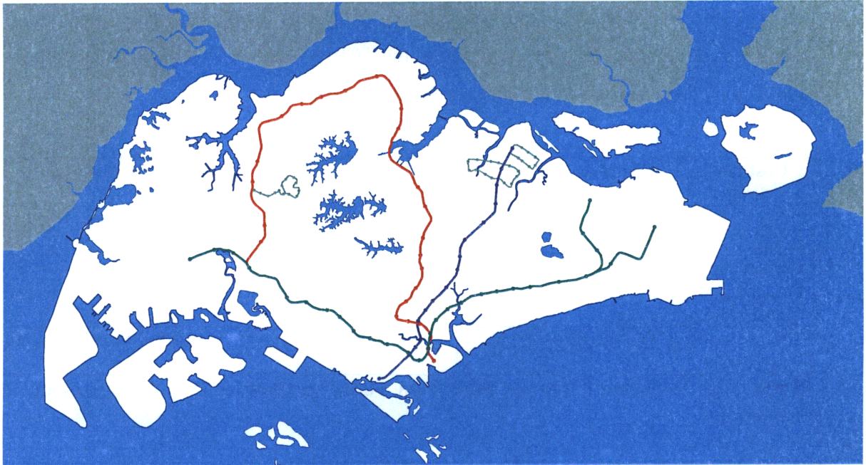
Figure 2.7: Singapore's RTS network. In red is the North-South Mass Rapid Transit (MRT) line, in purple, the North-East MRT Line, in teal, the East-West MRT line, and in grey, the Light Rapid Transit (LRT) lines serving local neighborhoods.
