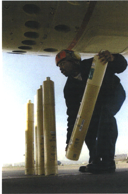
Figure 1-1: A U.S. Navy sailor loads DIFAR sonobuoys onto a P-3 Orion aircraft. [13].
