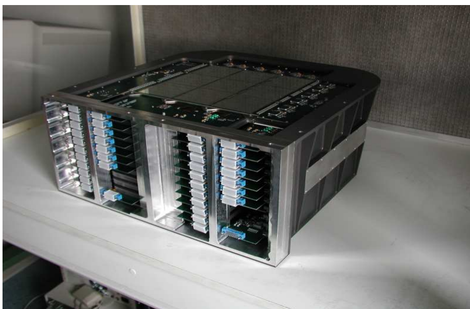
Figure 5. The PAMELA calorimeter flight model.
