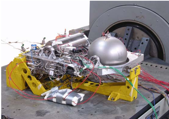
Figure 6: Box S engineering prototype and test fixture (yellow) mounted on slip table
