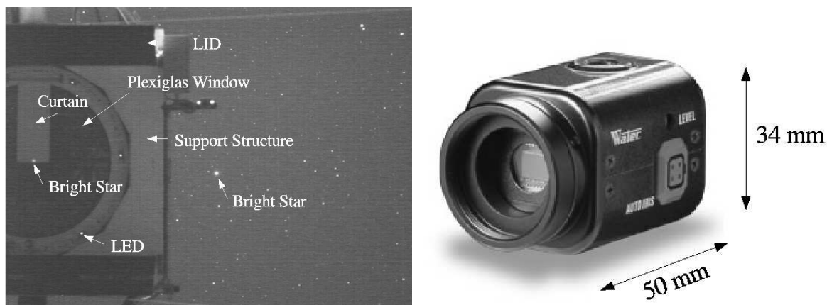
Figure 1. Left: Display window of the tracking monitor. With the three LEDs mounted on the PMT-camera frame a calibration is possible. To visualise the image of the bright star reflected from the main mirror to the PMT-camera a curtain was attached. Right: CCD-camera Watec WAT 902H
