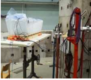
Fig.4: Ice block installed in front of a proton beam at TSL Uppsala
