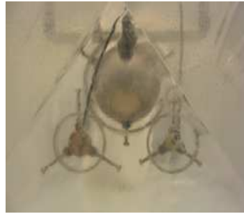
Fig.2: Sensor installation seen through \sim 1 m of clear ice
