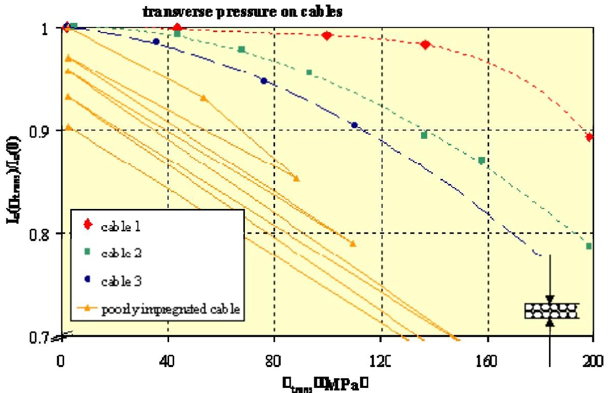
Fig. 5 Typical reduction of the normalized critical current of 3 different Nb<sub>3</sub>Sn cables under transverse pressure @ 11 T, 4.2 K. At pressures above 160 MPa permanent I<sub>c</sub> degradation occurs for most cables. Also shown is the behaviour of a cable which lacks of complete resin penetration inside the cable.
