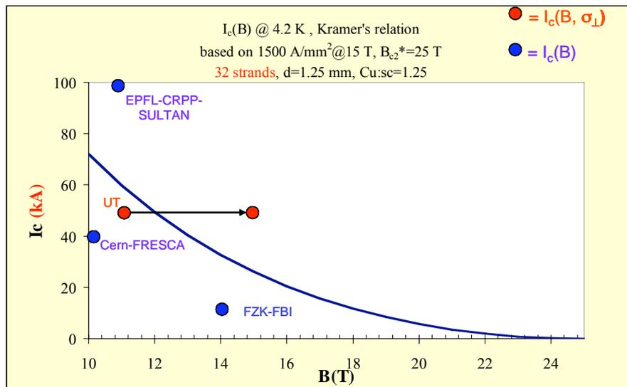
Fig. 6. Expected  $I_c(B)$  values for the proposed NED cable. Also shown are the measuring capabilities of existing facilities in Europe for cable measurements.
