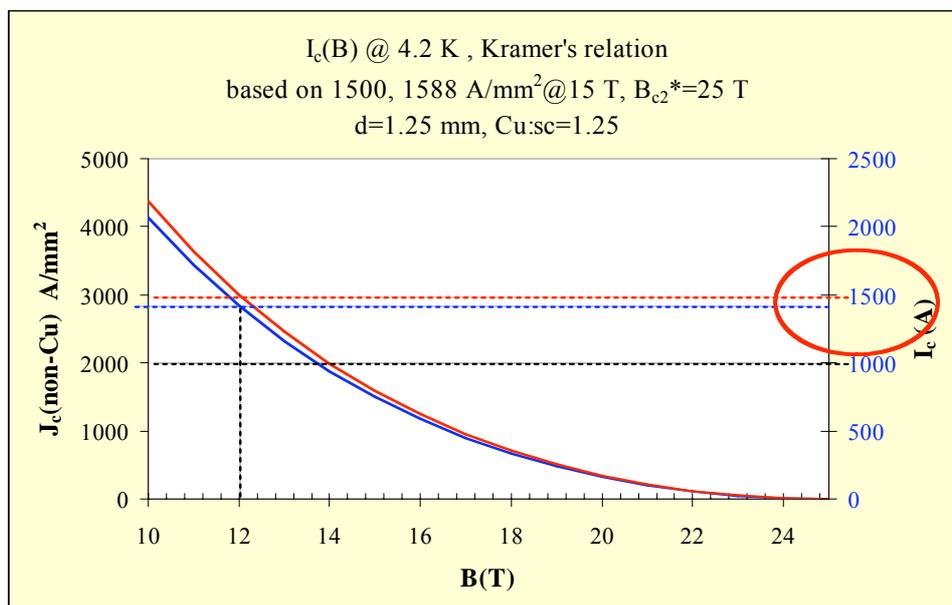
Fig. 3 Expected  $I_c(B)$  at 4.2 K of a 1.25 mm Nb<sub>3</sub>Sn wire in the NED program with a non-Cu  $J_c$  of respectively 1500 and 1588 A/mm<sup>2</sup> @ 15 T.
