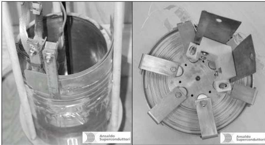
Fig.7. Solenoid and pancake coil (Ansaldo Superconduttori, Genova)
