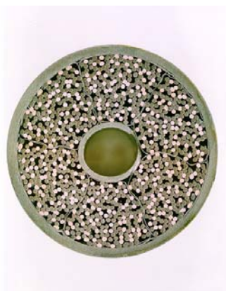
Figure 3: TFMC conductor ( \Phi=40.7 mm)
