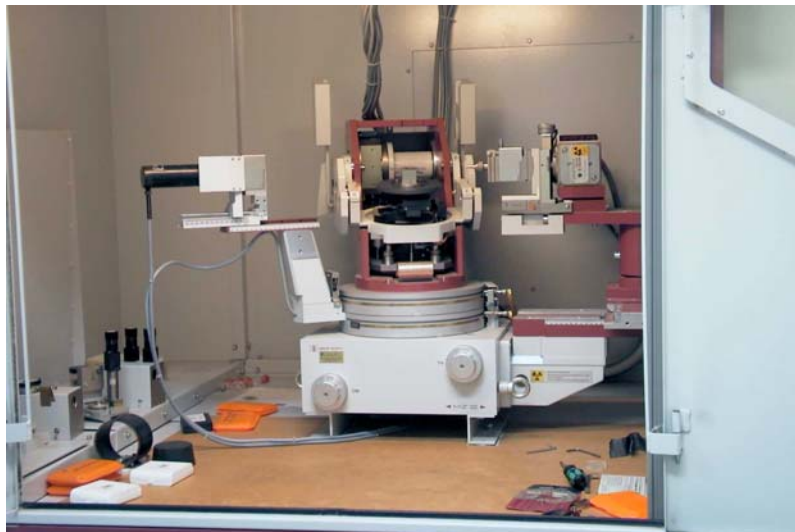
Fig. 1: the SEIFERT diffractometer with a four circle goniometer.
