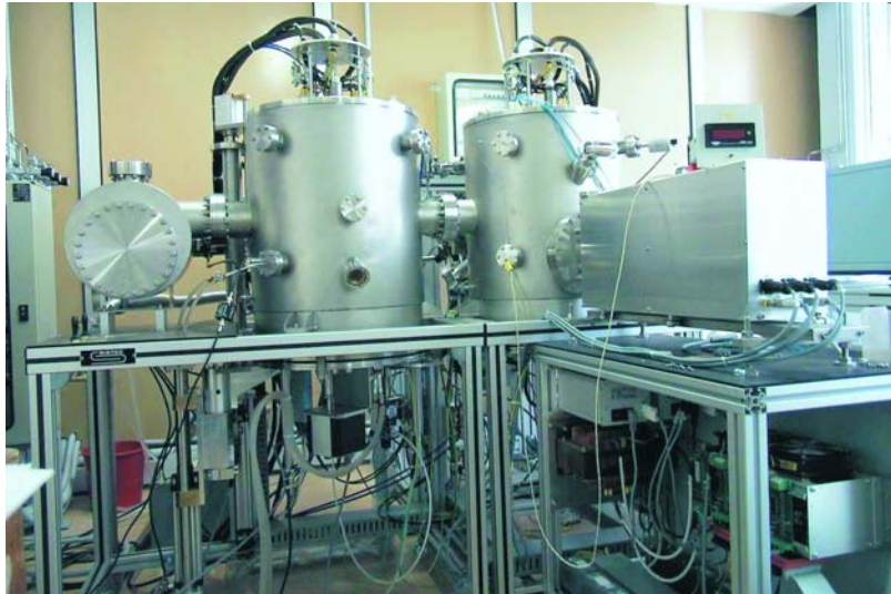
Fig. 4: the ENEA plant for continuous deposition of YBCO-based coated conductors.
