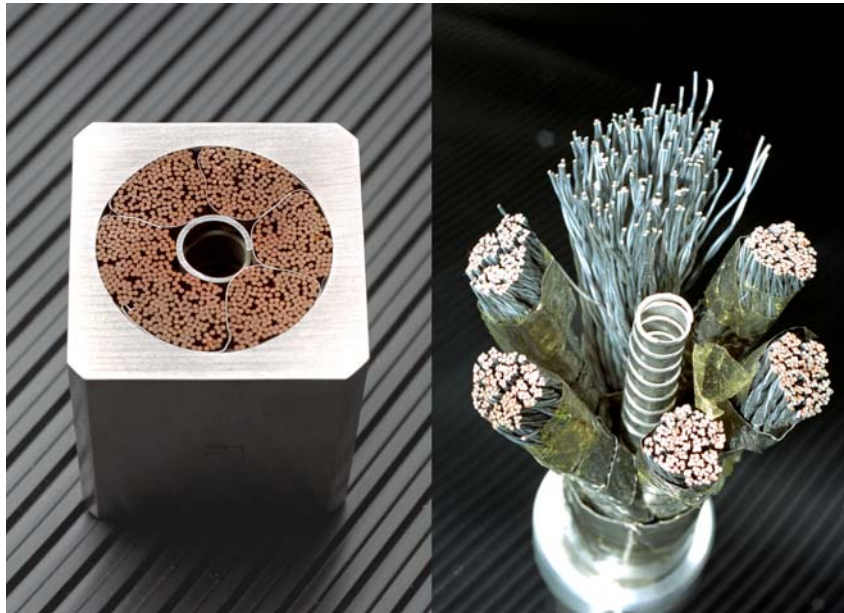
Fig. 10: picture of a section of the full-size Cable-in-Conduit Conductor adopted for the ITER magnets. External jacket dimensions are about 50 mm x 50 mm.
