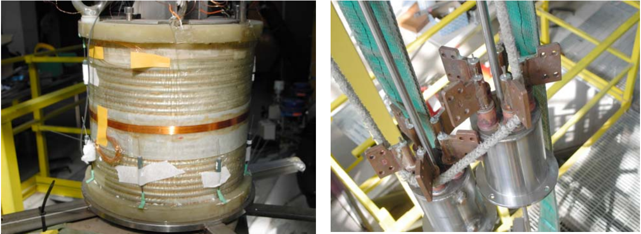
Fig. 6: the instrumented ASTEX module and its terminations, at which the cable has been opened and subdivided.
