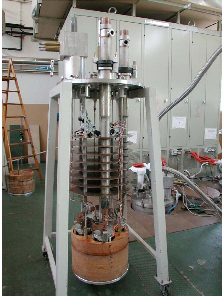
Fig. 11 : Cryostat insert with four mounted diode stacks ready for testing at ENEA laboratory.
