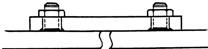
c. Stud weld bolts on the structure and then securely fasten the cover plate work holes by nuts
