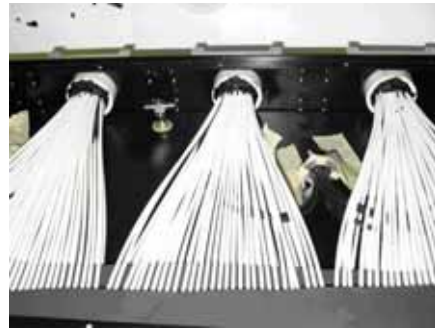
Figure 1. Photograph of hodoscope clear fibers and aluminum cookies.
