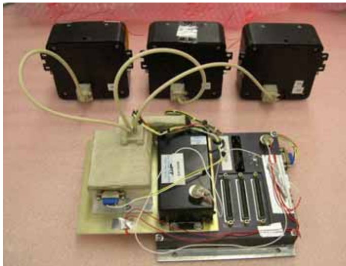
Figure 2. Hodoscope readout setup with Motherboard box, HVPS and 3 HPD boxes
