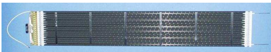
Figure 2. An AMS TRD straw tube module
