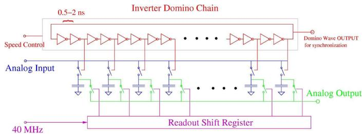
**Figure 1.** Schematic picture of the Domino sampler. Shown on top is the inverters sequence that originates the Domino wave. The shift register on the bottom enables serially the single capacitors connecting them to the output stage.
