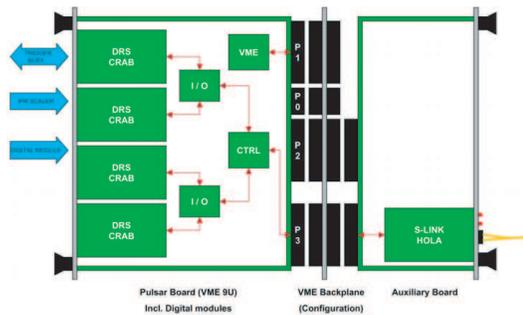
**Figure 3.** Schematic drawing of the data readout board.
