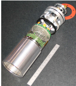
Figure 1. Hermetic PMT housing.
