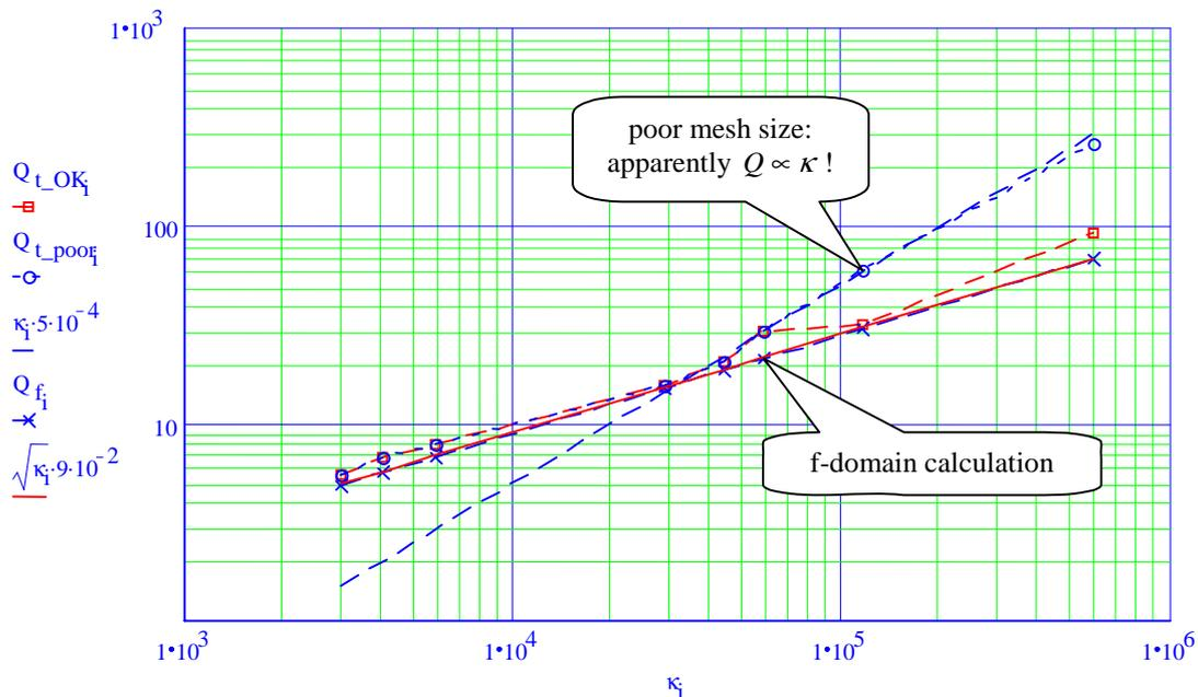
Figure 8:  $Q$  values calculated for different conductivities, comparing time and frequency domain data
