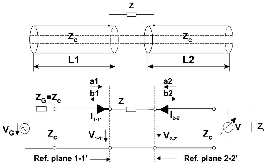
Figure 2: S-parameter measurement set-up for a single lumped impedance
