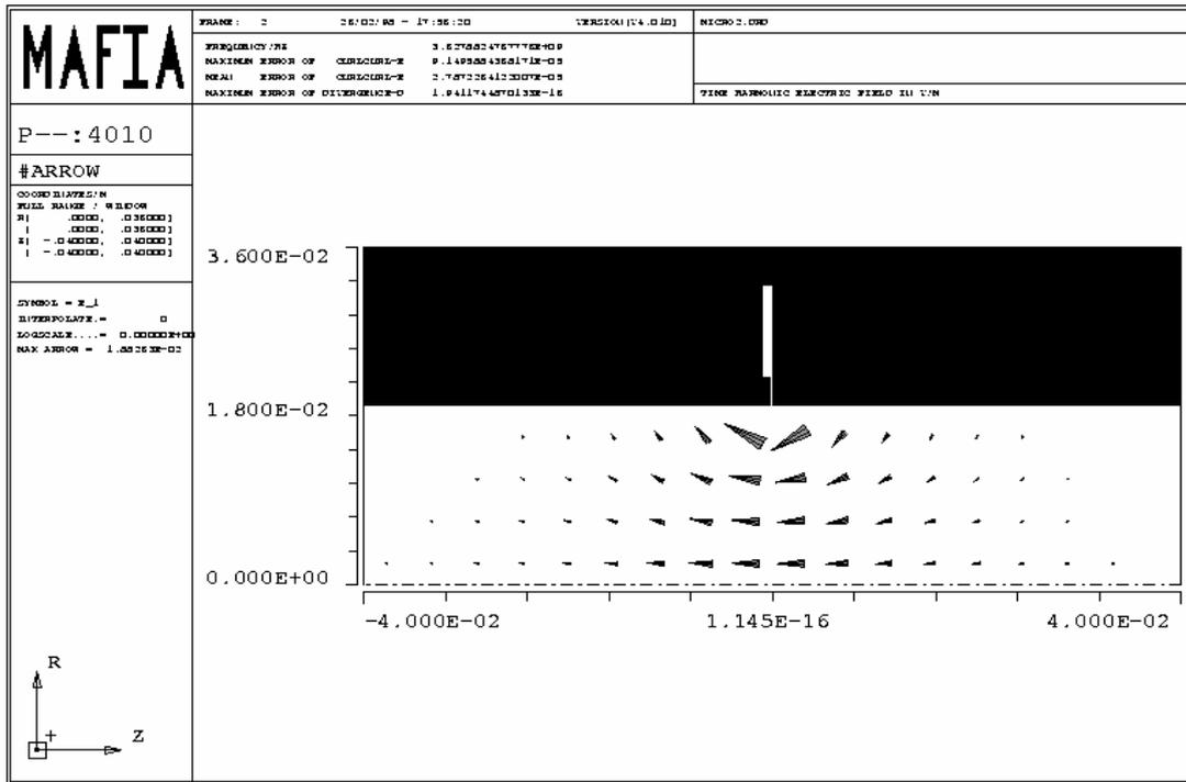
Figure 5: Electric field [V/m] of the fundamental mode near the gap.
