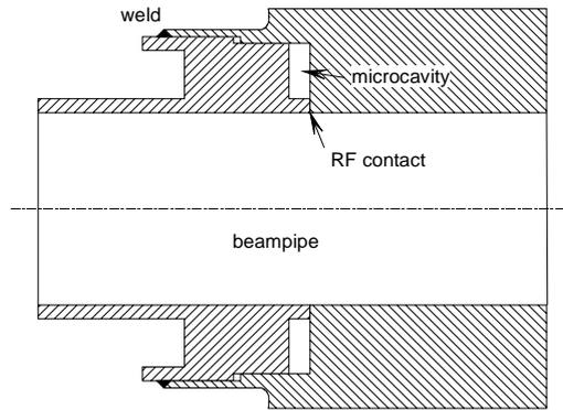
Figure 1: Beam pipe connection
