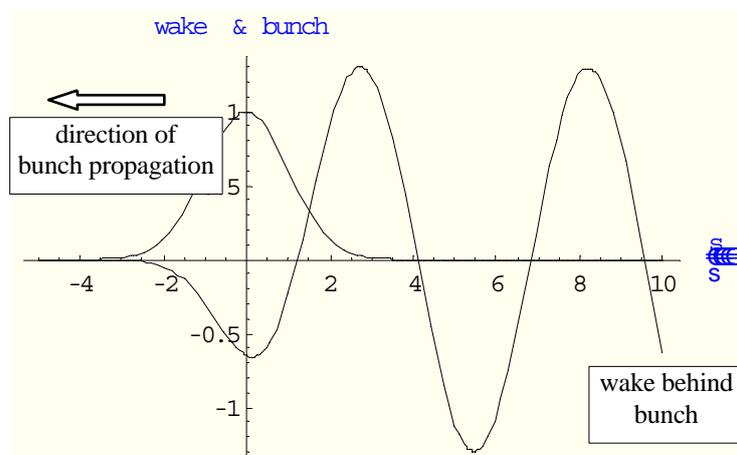
Figure 4: Typical longitudinal wake potential of a Gaussian bunch
