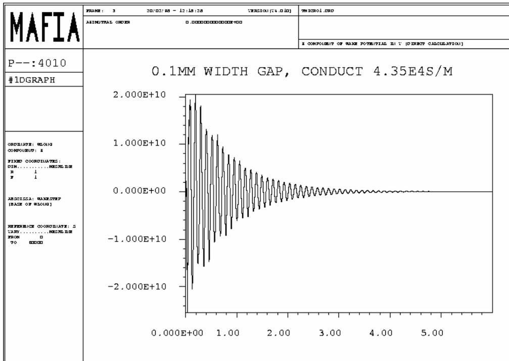
Figure 6: Wake potential [V] in the beam pipe vs. distance  $s$  [m].
