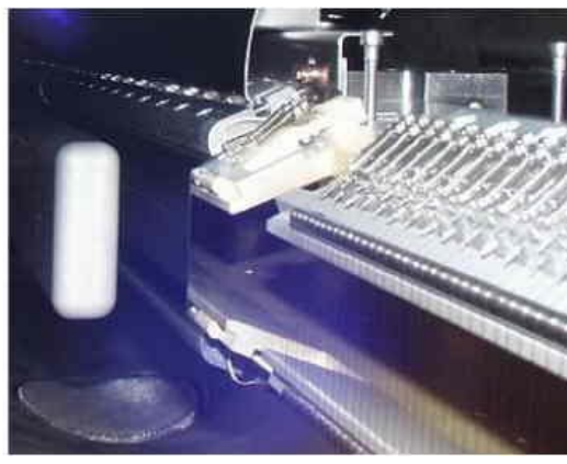
Figure 1: Relevant Geometry. The left picture shows the inside part of the septum tank with the nearly elliptical septum C-support and the wires. Pumping holes are visible in the right part of the pipe. The right picture shows an enlarged view inside the tank, close to the septum foil. The wires and the molybdenum foil are separated by a slot.
