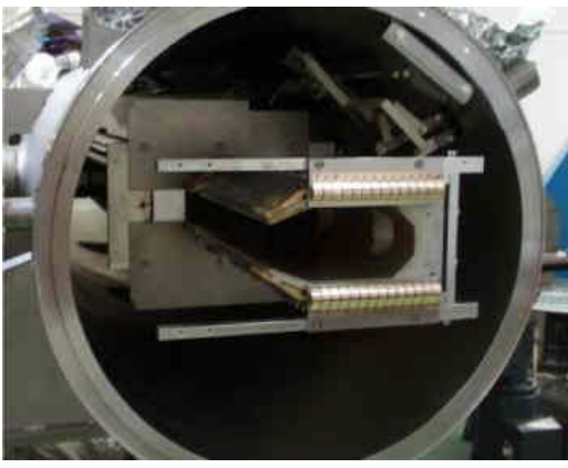
Figure 1: Relevant Geometry. The left picture shows the inside part of the septum tank with the nearly elliptical septum C-support and the wires. Pumping holes are visible in the right part of the pipe. The right picture shows an enlarged view inside the tank, close to the septum foil. The wires and the molybdenum foil are separated by a slot.
