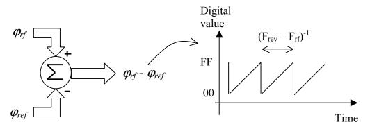
During acceleration the value of  $\varphi_{ref}$  and  $\varphi_{rf}$  is incremented at each clock cycle (the clock is supposed to be common). If reference and rf were at the same frequency, the output of the phase subtracting point would be constant. In the general case it will be a saw tooth with a repetition rate equal to the frequency difference.
