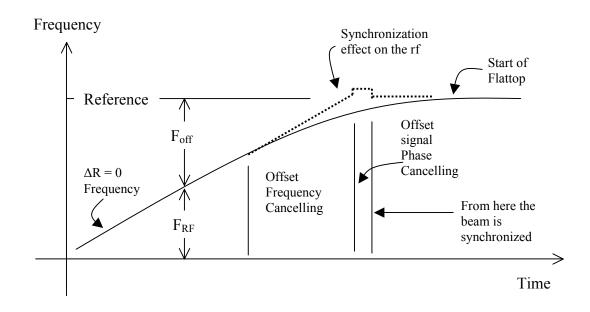
This graph defines the offset frequency  $-F_{off}$  - as the difference of reference and rf. The sum of rf and offset is called "moving reference" and can be compared (and locked) to the real reference anytime during the accelerating cycle.
