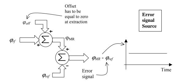
The error signal is now the difference of an extrapolated (or estimated) rf phase  $\varphi_{MR}$  (the moving reference phase) and the reference phase  $\varphi_{ref}$ . The principle is that the increment per clock period of  $\varphi_{off}$  plus the increment of  $\varphi_{rf}$  is equal to the increment of  $\varphi_{ref}$ . The resulting  $\varphi_{MR} - \varphi_{ref}$  is thus constant during the accelerating cycle. This trick enables the synchronization loop to be closed at any time.
