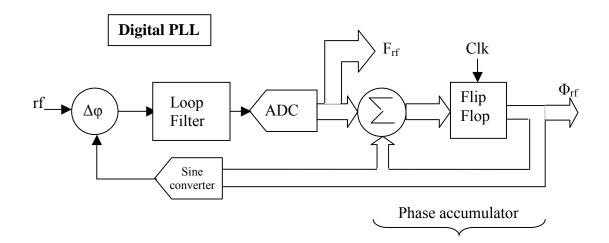
This simplified figure shows how the frequency and phase words can be extracted from an analogue rf signal. The rf is fed into a phase discriminator where it is compared to the phase word  $\varphi_{rf}$  reconstructed into a sine wave.
