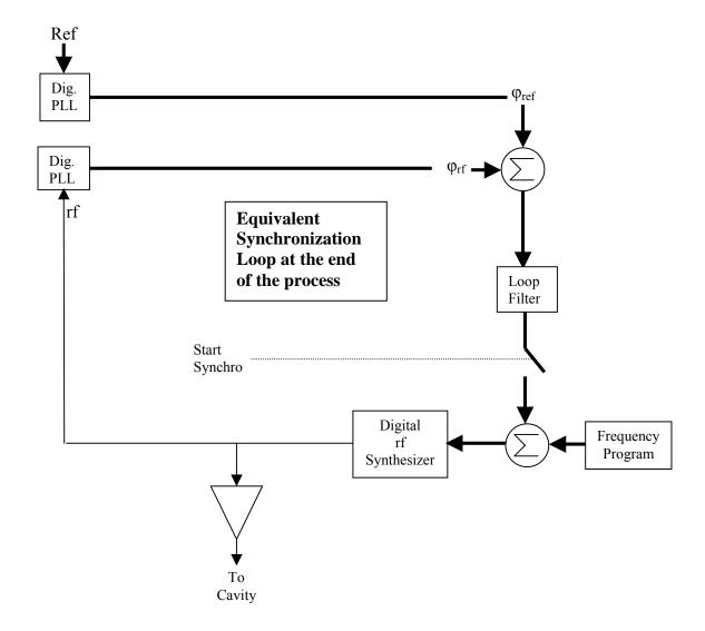
When the moving reference has been forced to zero, the equivalent loop diagram is typically of a classical type. The only novelty is the digital Phase Locked Loop from where the phase value is obtained as a binary word.
