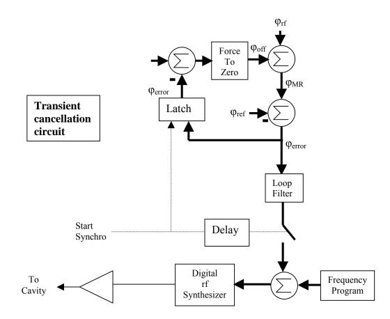
After being closed smoothly, the synchronization loop should have no effect on the main phase loop as the error signal is kept to zero by the very manner the moving-reference is created (feed forward process). It can be interpreted as a zero gain loop.
