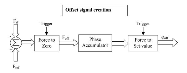
This diagram shows that  $F_{off}$  is obtained by subtracting reference and rf frequency words. A phase accumulator is then creating  $\phi_{off}$ . Note the presence of two "force to zero" boxes; their function is essential as the moving reference is to become null at the end of the synchronization process. Instead of null,  $\phi_{off}$  may as well settle down to a constant setvalue to change the synchronization phase. This explains the "force to set value" box.
