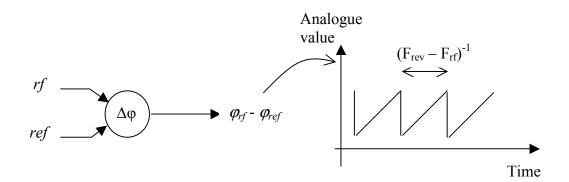
In the new system, same thing! The slight difference is that, instead of the rf analogue signals, we compare the digital phase values of rf and reference. The digital phase value of an rf signal is typically available at the output of a phase accumulator in a digital synthesizer.
