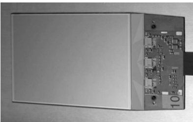
Figure 7. An IT module with one silicon sensor. The silicon sensor is 7.8 \times 11\ \text{cm}^2 in size. The three Beetle front-end chips are glued to the kapton hybrid and wire bonded to an Alumina pitch adapter.
