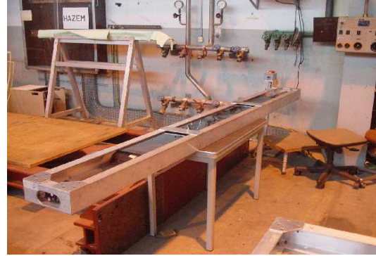
Figure 2. An ACORDE module; the scintillator modules consist of two superimposed scintillator counters.
