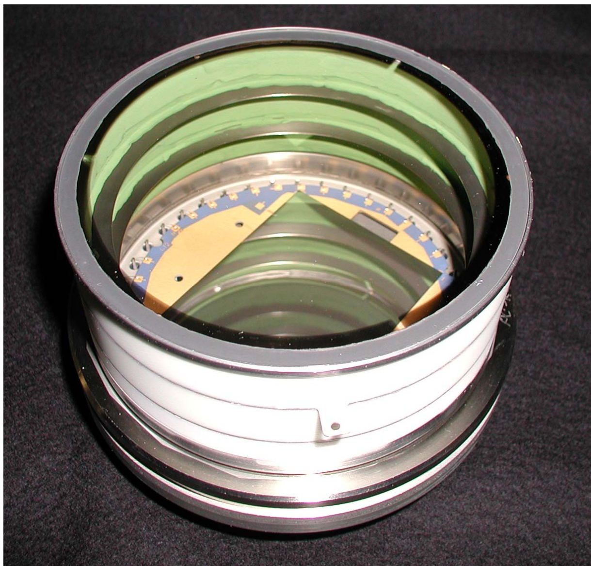
Figure 3: Photograph of the sealed PET-HPD prototype tube. The Al-coated Si sensor is clearly visible.
