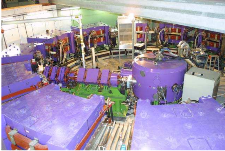
Fig. 4: The 150 MeV scaling FFAG built at the KEK laboratory in Japan
