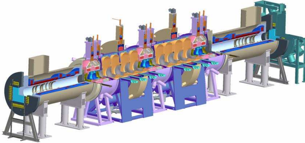
Fig. 2: Drawing of the MICE experiment [9]. The beam enters the experiment from the bottom left-hand corner. The beam first passes through one of the scintillator hodoscopes that form the time-of-flight system. After passing through the upstream spectrometer, the beam passes through three absorber/focus-coil modules and two cavity/coupling-coil modules before it passes through the downstream spectrometer and, a second time-of-flight hodoscope, the downstream Cherenkov counter and is stopped in the electromagnetic calorimeter. The beamline and upstream instrumentation is not shown.
