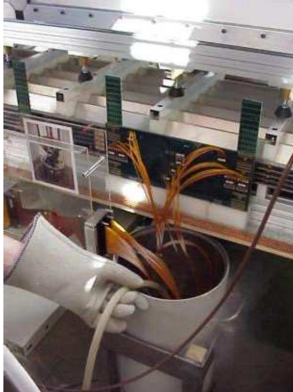
Figure 5.10: Calibration-injection and signal-readout cables, kept in a \text{LN}_2 dewar from the MB connection up to the warm-to-cold pin carrier.
