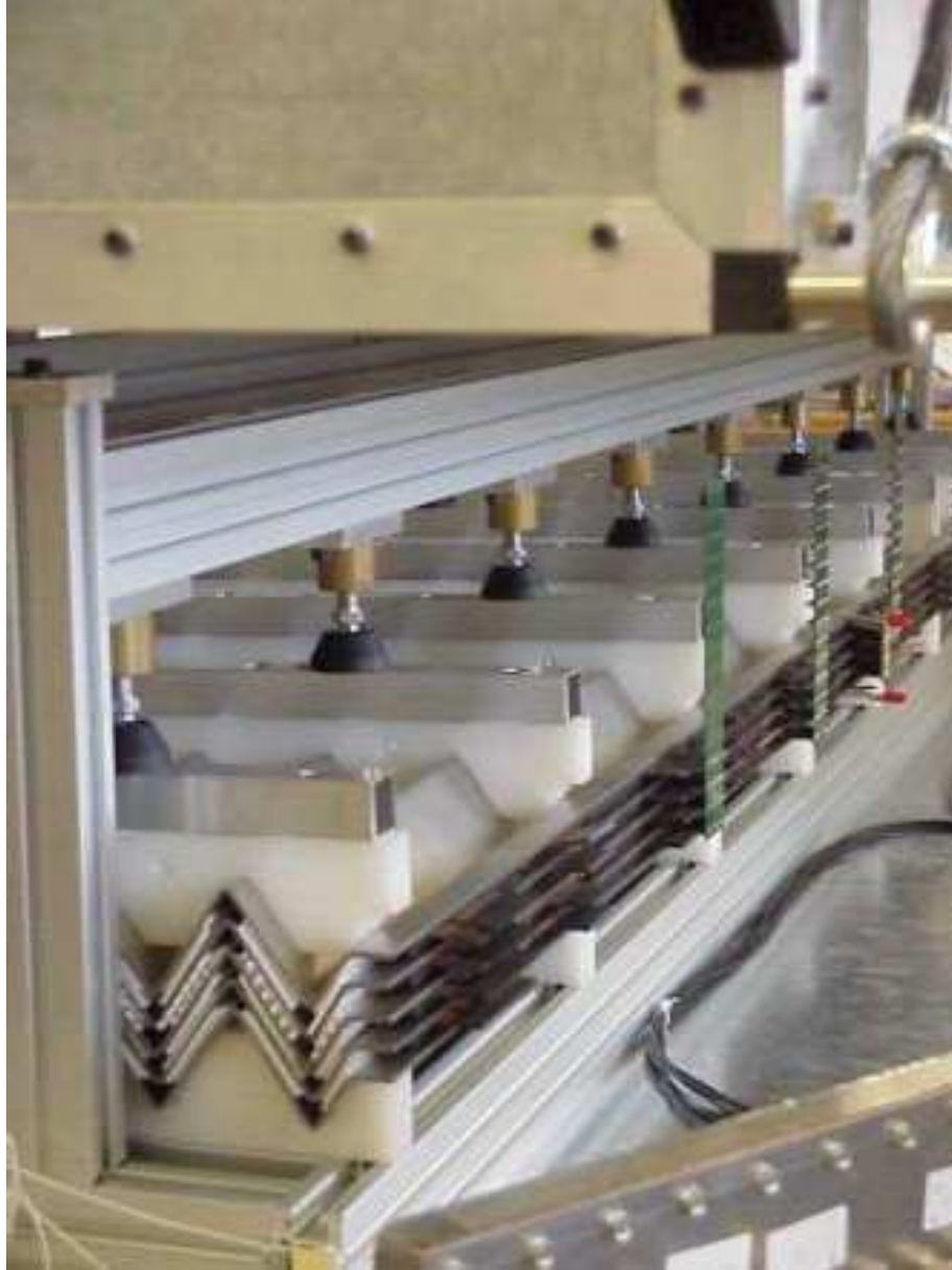
Figure 3.5: Detail view of the mock-up system in its final layout; the accordion structure of the detector is visible.
