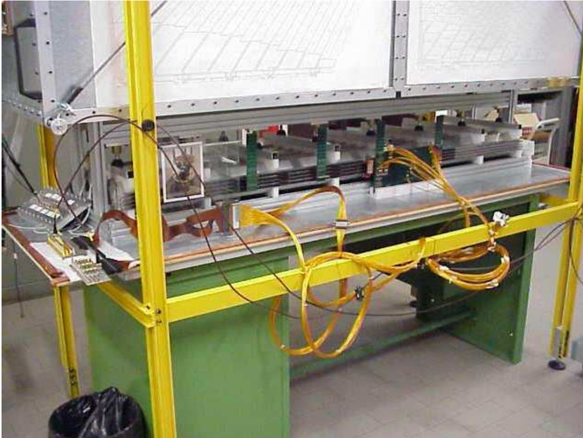
Figure 5.9: Mock-up system setup, complemented with the full calibration-injection and signal-readout cables chains.
