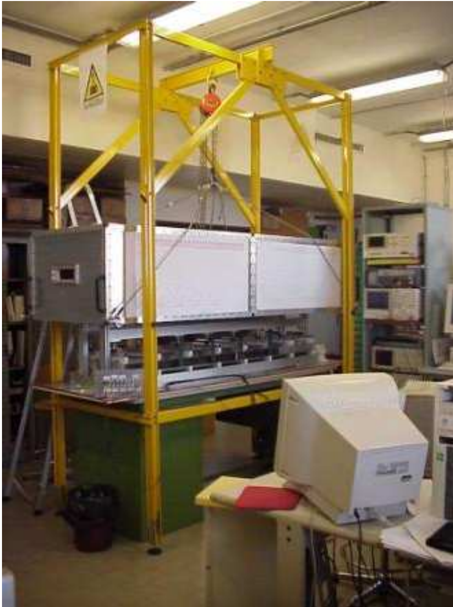
Figure 3.6: View of the mock-up system in its final layout; the Faraday cage is visible on top of the detector model.
