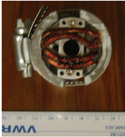
Fig. 8.12. Picture of the end turns impregnated with epoxy.
