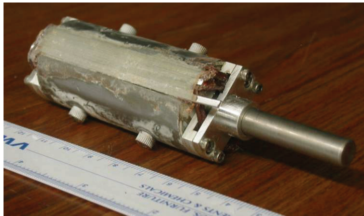
Fig. 8.14. SolidWorks ® model and picture of mold without clamping pieces.
