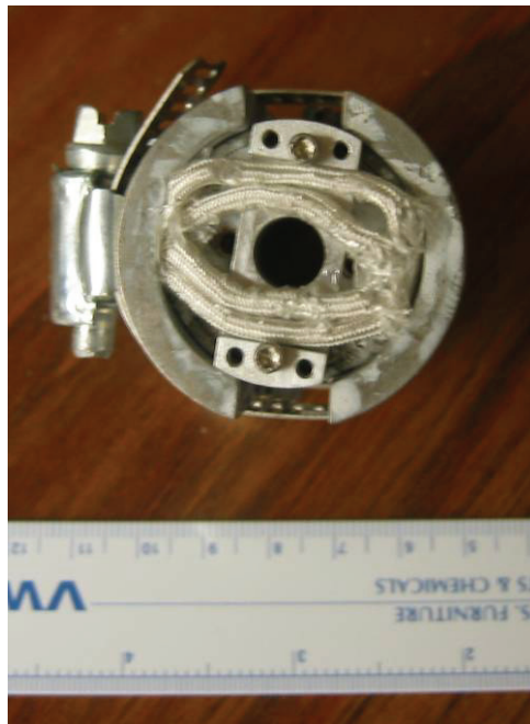
Fig. 8.11. Picture of the end turns in desired positions.
