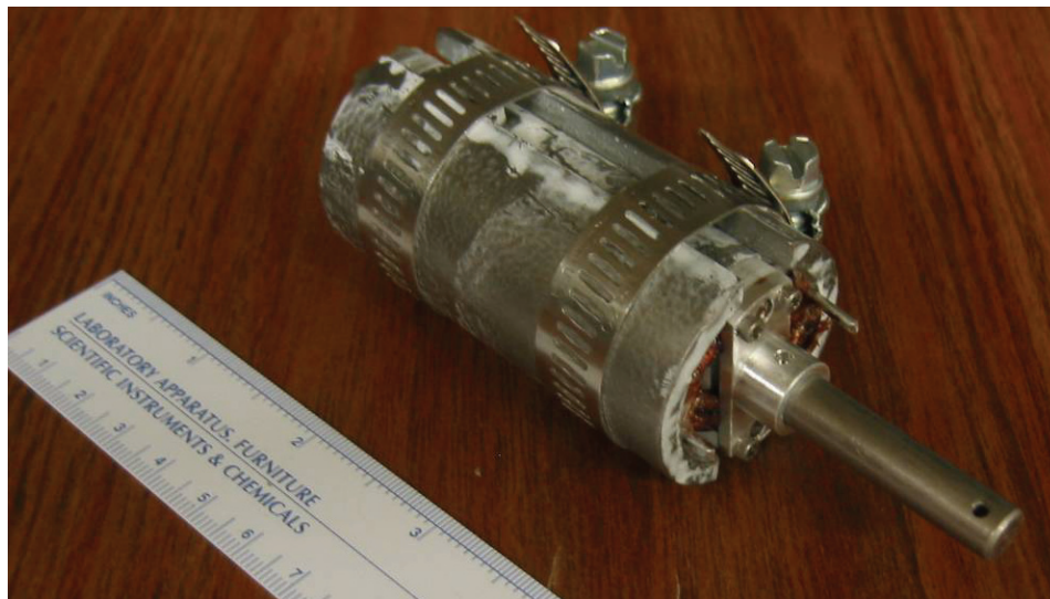
Fig. 8.13. Picture of the armature structure before curing.
