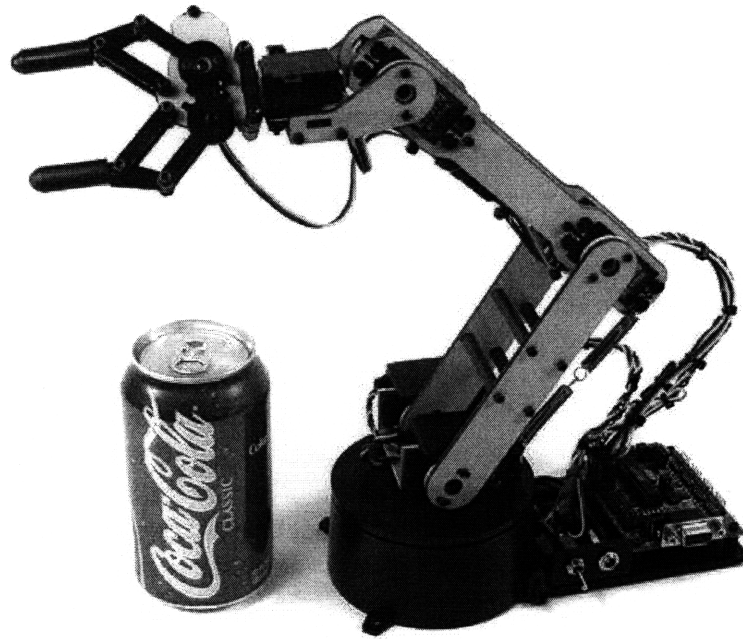
Figure 2. Lynx 6 created by Lynxmotion 9 is a commercially available robotic arm that has six degrees of freedom that can each rotate 180°.
