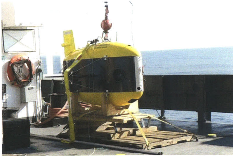
Figure 2-10: Odyssey IV at field operations in Georges Bank. The two main thrusters are controlled by a single rotating thruster unit, incorporating a brushless kit motor and resolver position sensor. This configuration allows high power vertical and forward motion with the same thrusters.
