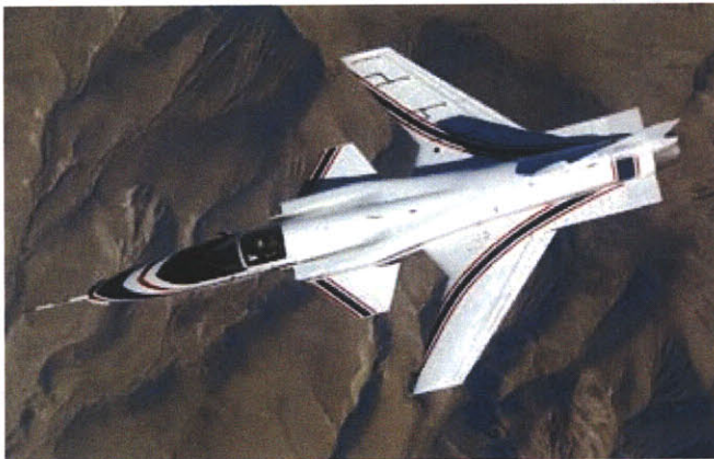
Figure 2-5: The X-29's unstable design requires a complex control system, but allows highly acrobatic maneuvers [29].
