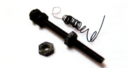
Example of SMA spring and screw fixture
