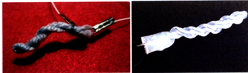
SMA and Teflon-wool spun yarn (left), and spun silicone and SMA strand (right)
