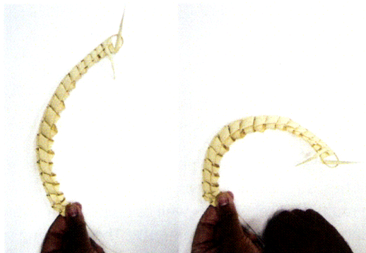
Javaé braided flexure: Pulling the strand at the bottom makes the braided structure curve
