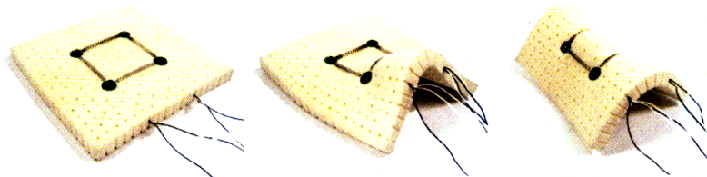
Surflex's surface deformation in three steps
