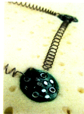
Detail of circuit board and SMA spring
