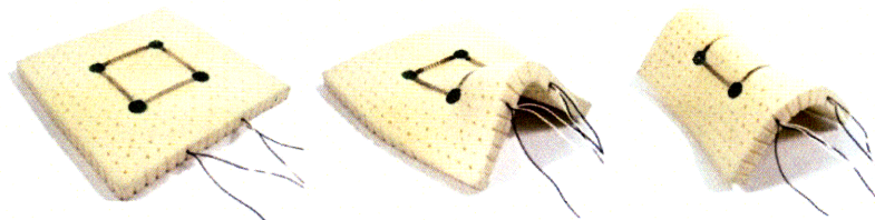
Surflex's surface deformation in three steps
