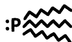
Figure 3-4: Chemical structure of trioctylphosphine. The unpaired electrons on the phosphorous atom passivate the surface of quantum dots.
