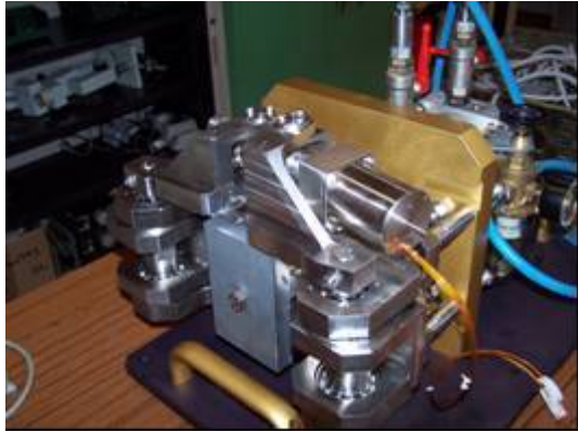
Figure 2: The measured stiffness on this test bench is 35 kN/mm. It is limited by mechanical plays in the ball bearing housings.
