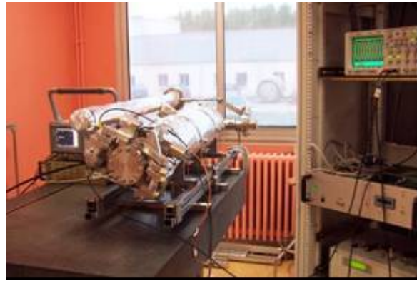
Figure 3: The piezo tuner is mounted on C45 TTF cavity with the electronics in the laboratory.
