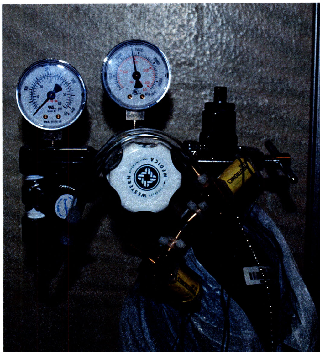
Figure 52: The USP oxygen cylinder, regulator and Parker valve
