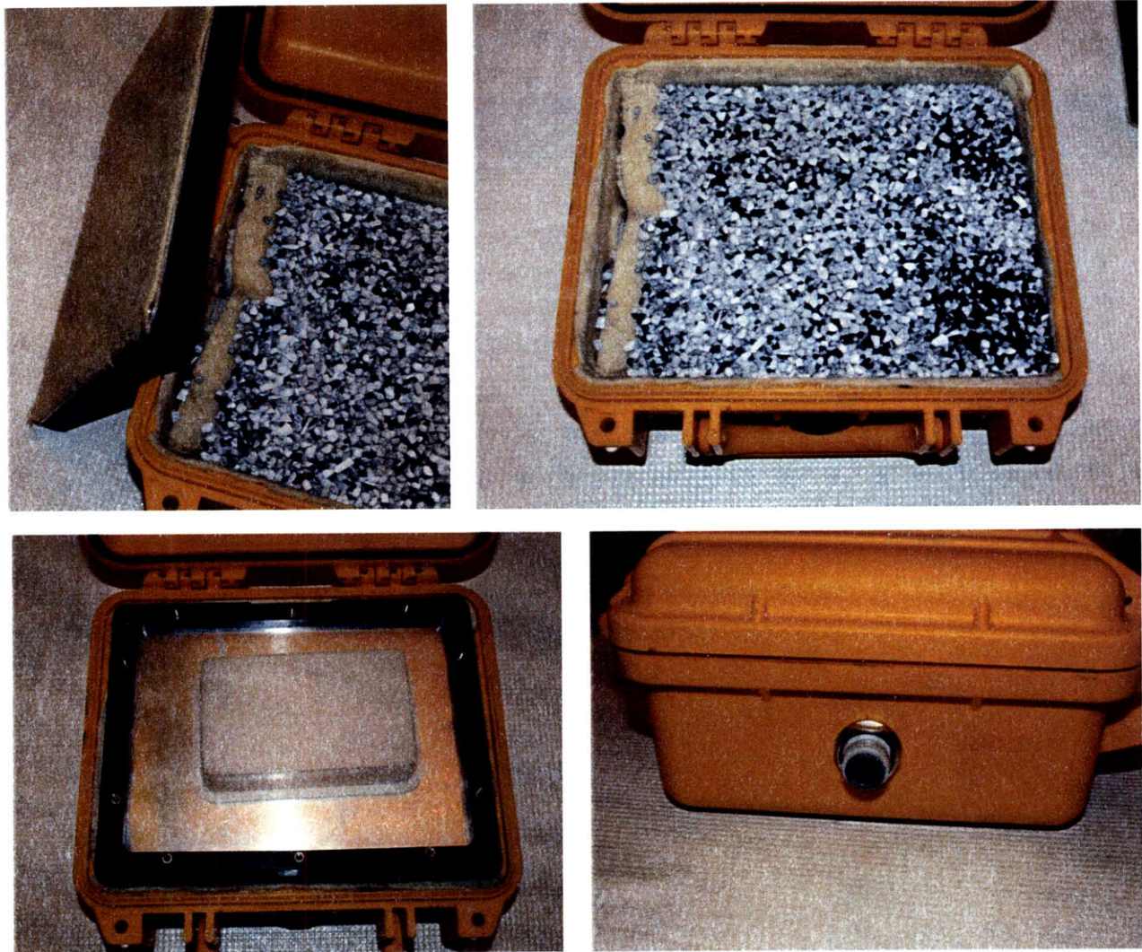
Figure 50: The IGTA ECLSS canister for LiOH and activated carbon
