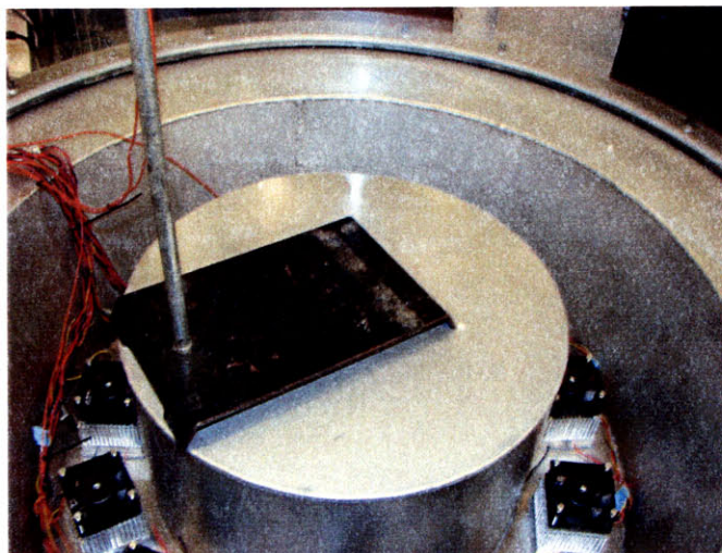
Figure 104: Impingement configuration units installed in the mockup
