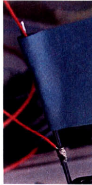
Figure 2-1: Fibers are contacted by wrapping a small wire around an exposed section of the core and applying silver paint. Such a connection is pictured here.
