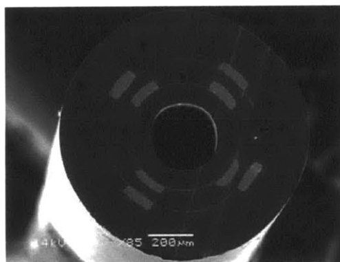
(b) SEM Image of two layer fiber. Credit to Dr. Fabien Sorin.
