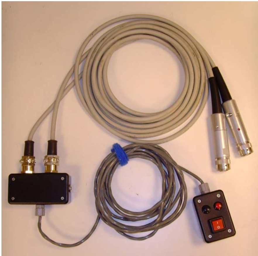
Figure 9 Custom switch unit built to operate two fluoroscopes simultaneously with a single input from the operator. Red and black buttons toggle high and low radiation dosage, respectively.
