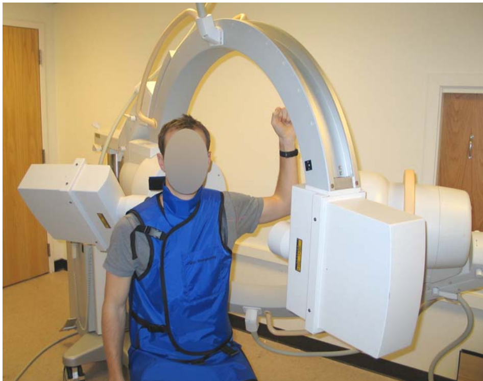
Figure 8 Dual plane fluoroscopic imaging system shown with a subject in the central viewing volume with the shoulder in 90° abduction with maximum external rotation.
