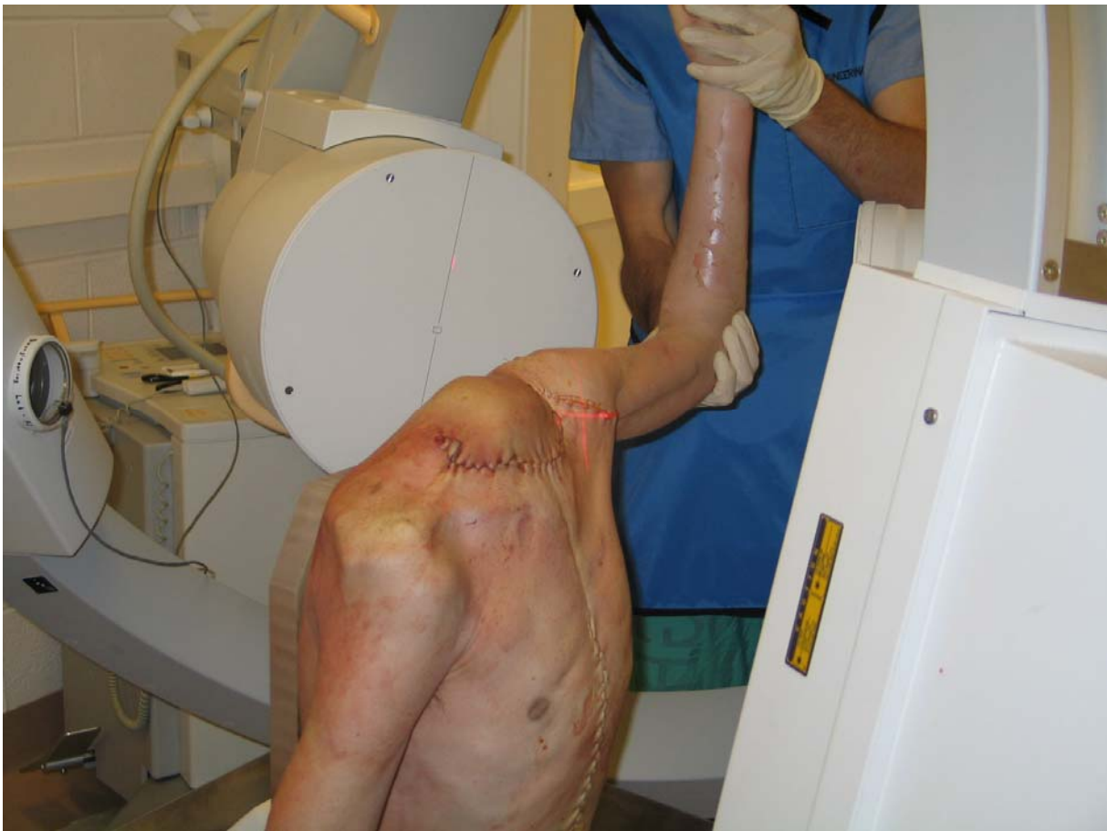
Figure 31 Cadaver rigidly mounted to a custom built fixture allowing the shoulder to freely move without obstruction. DFIS shown in image capture geometry.
