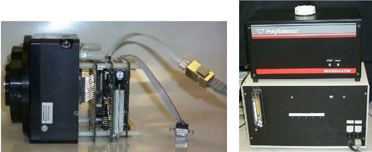
Figure 4: Photographs of the CID camera with the attached data acquisition cards and the “support package”, used for data integration and cooling of the chip.
