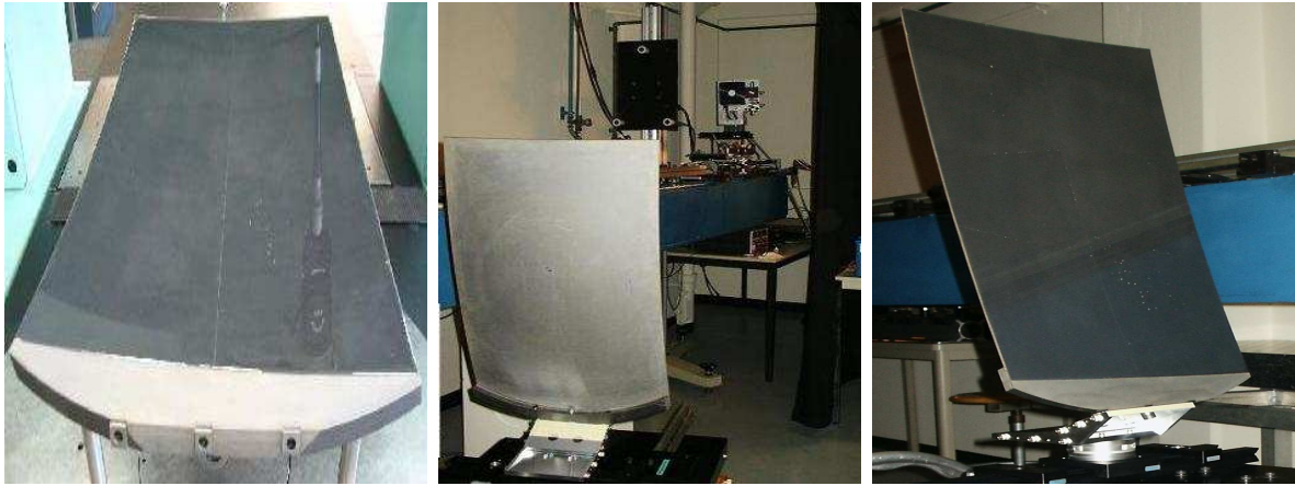
Figure 9: Three photos of the full-sized prototype mirror. Left, a view from above showing the glass coating (dark area) and the rim with the three holes. Centre, a back view of the mirror showing the grey beryllium substrate and the measurement setup. Right, a front view of the mirror showing the glass coating (dark area). In the centre and right photos, the mirror is supported by its rim from the bottom with a single bolt and tilted vertically by \sim 13^\circ for the D_o measurement under the effect of gravity.
