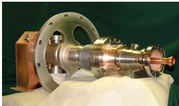
Figure 7. The AMAC coupler developed for TESLA/ILC.
