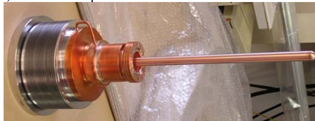
Figure 6. Proto-type of cylindrical window coupler for SPIRAL-II.
