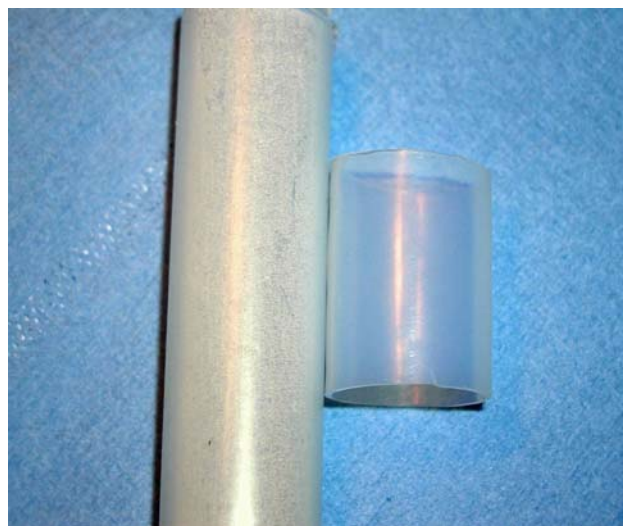
Fig. 7: Tube with sulfur layer and after ethanol cleaning
