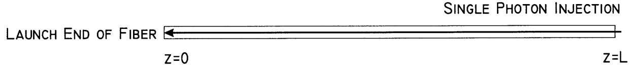
Figure 6-3: The SBS power at the launch end of the fiber can be calculated by injecting 1 photon per mode at z = L .
