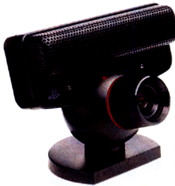
Figure 19 – The Playstation 3 Eye has a camera and microphone for audio and visual input, and can be used as a direct manipulation interface
