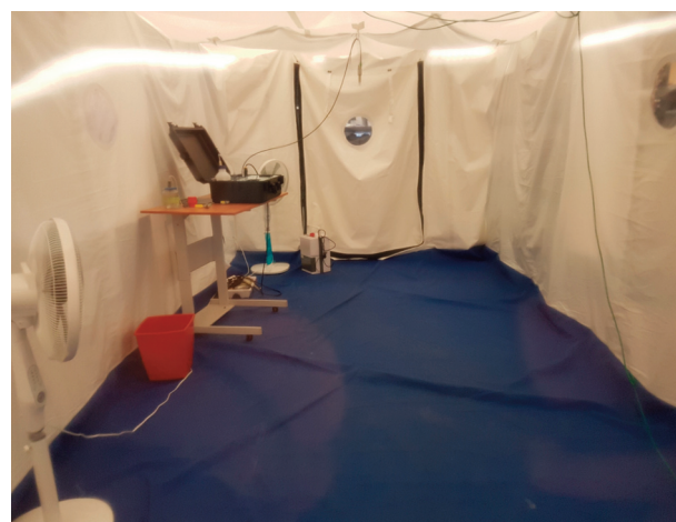
Fig. 2. The experimental enclosures used in the experiment: (a) one-cubic-meter stainless steel enclosure for online device testing; (b) the internal view of the larger 36 m 3 tent used on Cleamix Oy premises for long-exposure decontamination tests.
