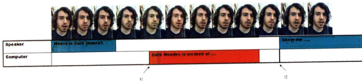
Figure 1-1: Diagram illustrating a speaker encountering a communication error. Notice that during the system’s conversational turn (from time t_1 to time t_2 ), where it is giving an erroneous reply, the speaker twitched his eyes naturally to signal an error. This suggests that visual analysis during the system turn may be useful.
